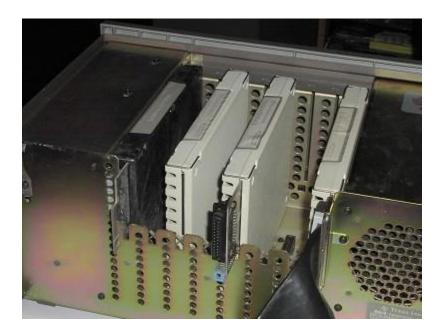
The first step is to remove the top cover, by pressing in the two clamps on the back of the PEB. This picture shows the cover removed from the PEB.
