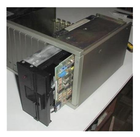
Slide out the floppy drive being careful to only pull it out far enough to reach the two connectors.
