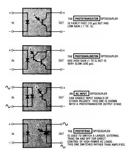
Most optocoupler use an LED as a light source. These are easily driven by most micro ports. Infrared light is used since its spectrum is more compatible with many light sensors and since you won't be watching it anyway. Almost all optocouplers are opaque packaged so that room lighting has no effect. As with any LED, you must be careful of the circuit polarity and must limit input current to a safe value, typically 10 milliamperes.
