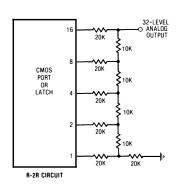
In the first circuit, we start with a CMOS port or latch and then add summing resistors that are weighted in a 1-2-4-8-16 ratio. These currents are summed to give an output stairstep voltage that has thirty-two levels. Note that the smallest resistor value gives the largest current, and vice versa.
