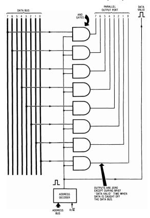
All we have done here is "insided out" the simple input port, putting the data bus on the left and the parallel output lines on the right. If these lines are the only thing going to the outside world, we may not have to worry about tri-state access, so we have shown plain old AND gates.
