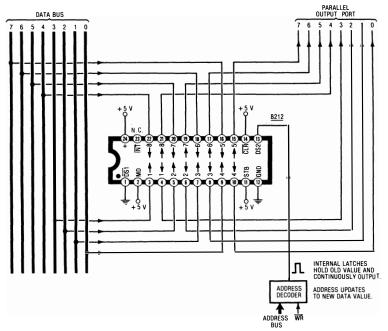
This time, the mode pin is positive. The mode pin changes the inside logic on the 8212. In the output mode, the address decoder decides when to update data into the internal hold-follow latches, and the tri-state drivers are continuously enabled by the high STB line.
