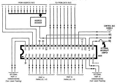
The port lines are arranged by eights into an A port and a B port. The supply power and system bus pins are connected the usual way. Four optional input or output lines intended for handshaking are called CA1, CA2, CB1, and CB2. These may be left unconnected for simple I/O uses.
