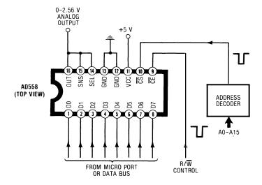
The way I have shown this circuit, you simply hang the *Analog Devices* AD558 on an 8-bit output port, and you get an output voltage of 0 to 2.56 volts that follows the straight binary coded inputs. All this from the same 5-volt supply the micro uses.
