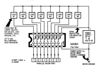
This octal peripheral driver comes in an 18-pin package and handles eight separate loads of up to half an ampere each, powered from an outside supply of 40 volts or less. The inside circuitry consists of eight separate Darlington transistor drivers, along with eight separate spike-protecting diodes. Once again, this supply *must* share a common ground with the microcomputer and the peripheral chip.
