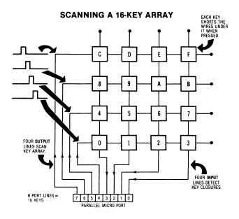
We use four output port lines and four input port lines. Only a single output line is allowed to go high at any instant. The output lines take turns going round and round as shown.
