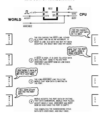
This time, the CPU checks to see if the port is still busy. If not, the CPU sends data by addressing the 8212. This latches data into the 8212 and drives BUSY and AVAILABLE low.
