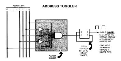
When you address the magic location, the output changes state. Address the location again, and the output changes once more, going from zero to one or vice versa. To output a square wave, you continuously address the magic location at *twi*ce the output frequency you want . . .
