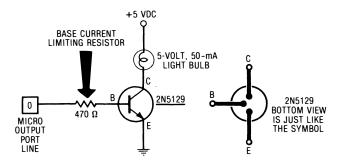
In this case, the lamp is the load for our NPN transistor. If the micro port provides a weak high output, this output in turn gives us transistor base current, turns the transistor on and saturates it, and puts nearly the full supply voltage across the lamp. This, of course, lights the bulb.
