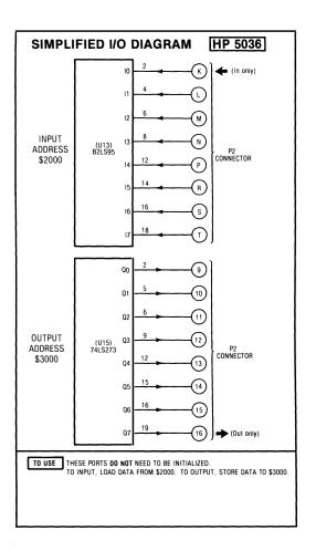
On this trainer, we have 8 input lines on top and 8 output lines at the bottom, both accessed via connector P2. Looking more closely, we see that input IO ("EYE-ZERO") enters the trainer via pin K of P2, and so on down the list.
