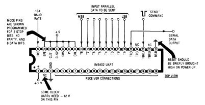
First you supply this 40-pin chip by putting  $\pm 5$  on pin 1 and grounding pin 3. This *Intersil* 6402 is a modern, single supply chip. Older devices may also want a  $\pm 12$ -volt supply on pin 2.
