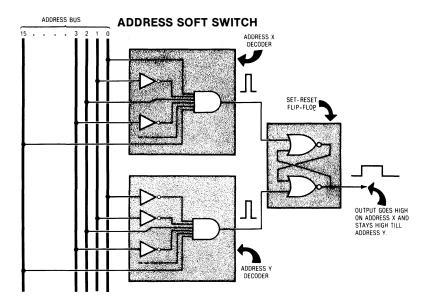
Here we have two decoders set to two different addresses. Address X sets a set-reset flip-flop and drives the output high. Address Y clears the set-reset flip-flop and drives the output low.
