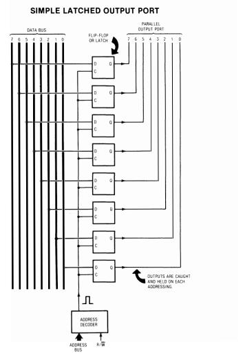
The address decoder works the same way as it did before. At the instant the address is valid, the data on the data bus is "caught" by the D-flops or latches and is then held. The output lines continuously output the data bus info saved during the last time the port was updated.
