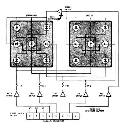
What you do is pick a non-obvious decoding. Note that the center spot is lit only on odd numbers. So, use one line as an
