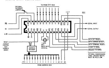
You power this chip from a single +5-volt source, and hook up the usual 6502 clock, reset, and R/W signals as shown. A 1.8432-megahertz crystal gets hung on pins 6 and 7 if you are using the internal baud rate feature. If you are using interrupts with your serial I/O, an IRQ output is connected to the  $\overline{\text{IRQ}}$  line in the micro system.
