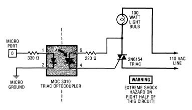
This circuit shows you how to let a microcomputer directly control a 100-watt light bulb connected to the AC line. In fact, the same circuit can be used to control up to 1000 watts of AC power if you use a fairly large heatsink on the big triac. The microcomputer port output lights the LED, which trips the little triac, which in turn trips the big triac. The big triac turns on and stays on till the main current through it drops to zero, as happens each AC half cycle.
