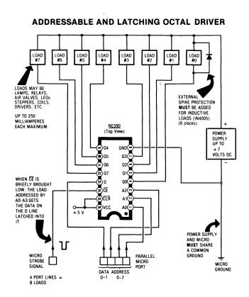
This one isn't quite as tough as the 2803. It allows only 200 milliampere loads at a maximum supply voltage of 7 volts.
