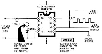
This special *Hewlett Packard* AC optocoupler directly and safely accepts a full strengh 110-volt AC line signal at its inputs by way of a large current-limiting resistor. This lights one or the other of the input LEDs, except during line zero crossings. The output of the optocoupler will go positive on each zero crossing of the AC line, giving you 120 pulses per second into your port. Extra goodies inside the chip improve the snap-action and stability.
